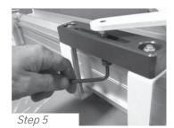
**STEP 5:** Remove the shoulder bolt that the fork pivots from.
