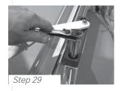
**STEP 29:** Tighten the two nuts with a  $\frac{1}{2}$ " socket wrench, ref. tighten to about 10' lb.
