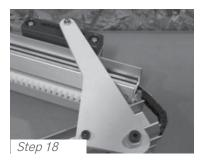
**STEP 18:** Line it up with your pencil mark and move the lift arm until the pivot aligns with the new position of the upper bracket.
