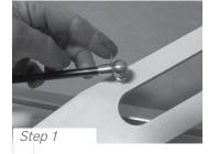
To remove the ball mounts, remove the wire retainer clips that hold them on. Pull the ball-ends straight-up to remove.
