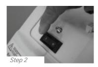
**Step 2:** Remove the safety tie and turn the red "ON/OFF" switch to the "ON" position (I).
