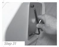
STEP 31: Use a <sup>5</sup>/<sub>16</sub>" Allen wrench to remove the two large bolts that hold the side-plate onto the Rave unit.
