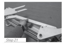
**STEP 21:** Position the link arm as shown at right between the tracks and the two pivoting arms.
