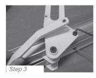
**STEP 3:** Catch the link and set it aside. Be careful not to damage the paint.
