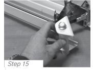
**STEP 15:** Slide the upper bracket off the upper track out of the open 'elbow.'
