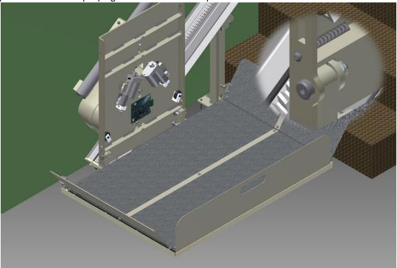
Fold the platform up and attach the ends of the assist struts using the clevis and cotter pins.
