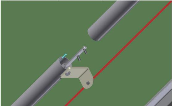
Secure the remaining guide rail mounting brackets to the rail with the threaded bars inside the rail channel. The bottom end of the guide rail should extend at least as far as the bottom end of the track. The upper end may be extended further so the guide rail can be utilized as a handrail for people traversing the stairs on foot.
