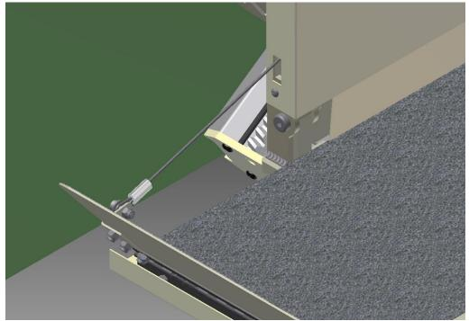
Insert the upper limit cam into the slot in the track at the top and tighten the set screw, this will need to be adjusted later to stop the lift in the proper location. Insert the rest of the gear rack into the top of the track. The gear rack should be even with the end of the track and the last piece may need to be cut off. Install the end plate using the four Torx head screws and Torx driver provided.
