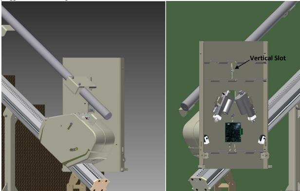
$Mount the \ Platform \ onto \ the \ lift \ using \ the \ shoulder \ bolts \ and \ nuts. \ \ Plug \ in \ the \ safety \ pan \ wire \ harness \ from \ the$
