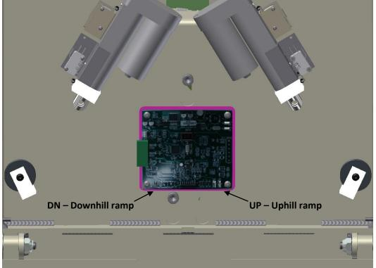
Plug in the harness on the shroud to the harness at the top of the platform mount. Route the two ramp cables through the two slots on either side of the shroud then secure the shroud with the four screws on the sides.
