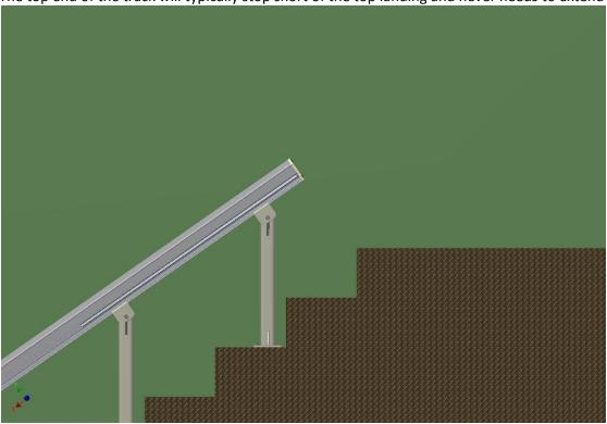
To mark the location for the upper guide rail measure from the leg base plate up the wall 36.25" (as indicated by the red vertical line). Make sure that you make this measurement in the center of the leg and that your measurement is plumb vertically. A 3 or 4 foot level will help ensure this.
