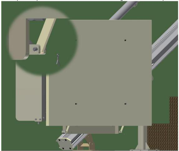
On the back side of the platform are two leveling bolts. Loosen the jam nut on each and turn the bolts in or out to position the platform. When empty the edge furthest away from the chassis should be slightly (1/2" - 3/4") higher to compensate for the deflection when fully loaded with a passenger and chair.
