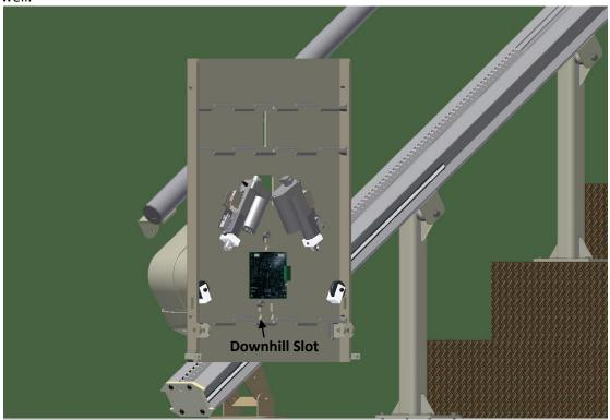
Install the Upper Guide Roller on the back side of the platform mount. Align the two wheels with the guide rail and secure with a washered bolt through the vertical slot in the platform mount. Plug in the three wire harnesses from the platform mount to the top of the chassis. All three plugs are different so they cannot be plugged into the wrong connector.
