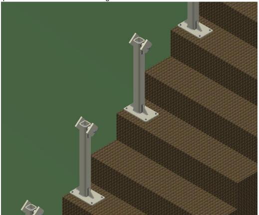
Set the lower section of track into the mounting legs. The clamps fit into a small channel on the bottom of the track. Do not fully tighten the clamps at this time.
