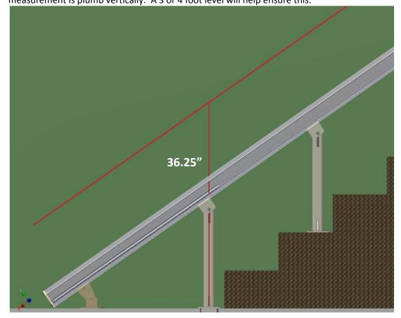
Repeat this measurement at one more leg at a minimum. Then mark a straight line between these measurements. If needed, a chalk line can be filled with talcum powder so there is no risk of discoloring the wall with standard chalk or pencil line.
