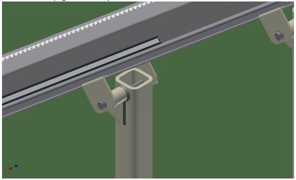
If your lift has multiple track sections, splice them together using the supplied splice bars and screws. The alignment pins will come pre-installed in one of the track sections. Before sliding track sections together be sure to plug together the charge wires running inside the track. After tightening the splice bar screws slide down the sections of goar rack so there are no gaps.
