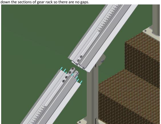
Position the track and mounting legs on the stairs until the desired dimension is obtained from the nose of the steps to the underside of the track. This dimension is noted on your specific installation drawing. The bottom end of the track should be no more than ½" off the floor and there is a short leg to secure the bottom. After ensuring the track is in the proper location, anchor down the legs with the four #14 wood lags provided with each leg.
